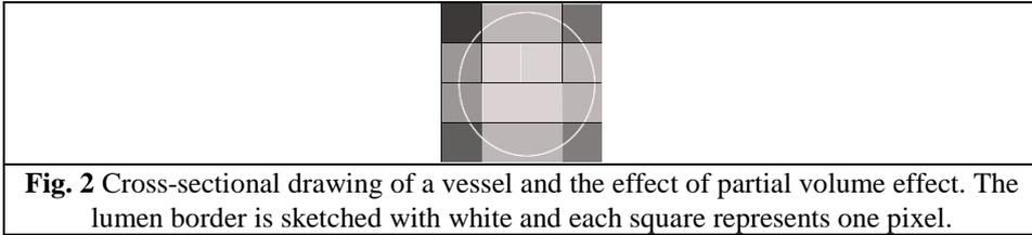
**Fig. 2** Cross-sectional drawing of a vessel and the effect of partial volume effect. The lumen border is sketched with white and each square represents one pixel.
